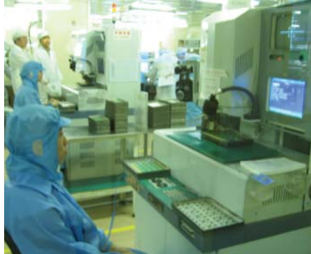
Quality Control using Automated Test Equipment in a Clean Room Environment
